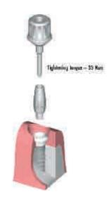
Important: For tightening the basal screw, the ratchet (Art. No. 046.119) with attached torque control device (Art. No. 046.049) and an SCS screwdriver
